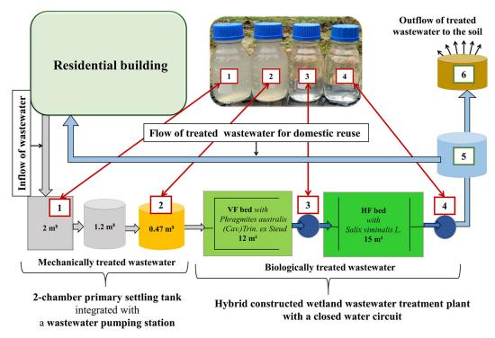
**Figure 3.** Schematic of the closed water circuit hybrid constructed wetland serving the employee housing unit in the PNP, Kulczyn, Poland. Wastewater sampling sites: 1 – primary settling tank (raw sewage); 2 – pumping station for mechanically treated wastewater; 3 – collection/distribution well downstream of the VF bed; 4 – collection/distribution well downstream of the HF bed, 5 – pumping station for purified wastewater; 6 – dry well – receiver of excess treated wastewater.
