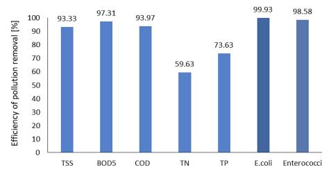
**Figure 9.** Average pollutant removal efficiency of the investigated CW in the start-up period. TSS – total suspended solids,  $BOD_5$  – biochemical oxygen demand, COD – chemical oxygen demand, TN – total nitrogen, TP – total phosphorus, E. coli – *Escherichia coli, Enterococci.*
